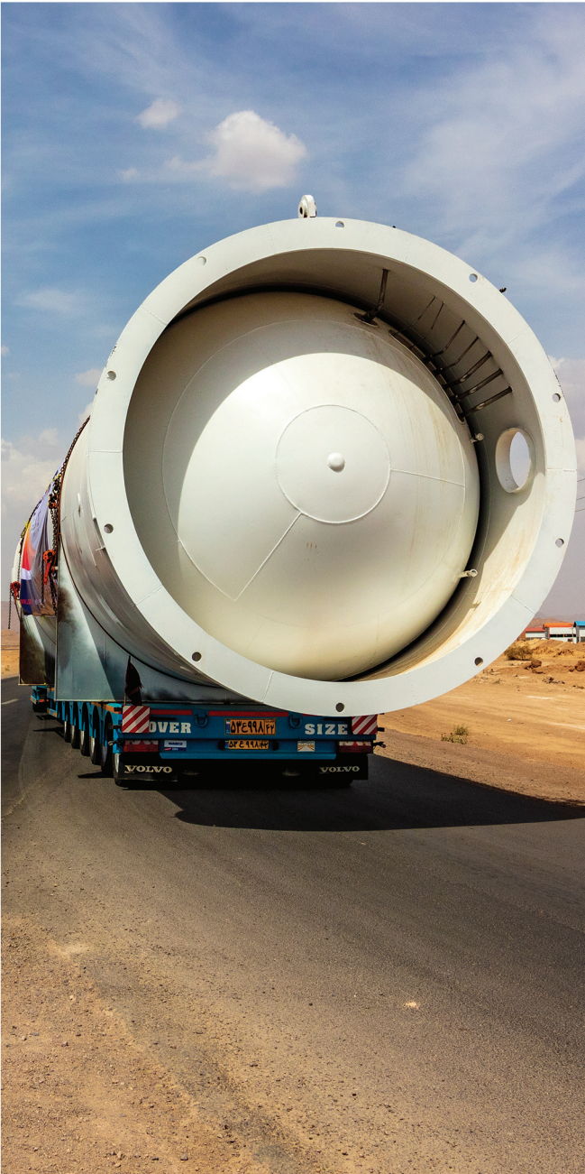
200m 3 Cryogenic Vacuum insulated tank
